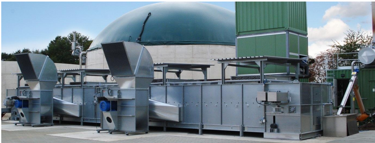
Figure 44: Belt dryer for digestate drying in front of a biogas plant (Source: STELA Laxhuber GmbH)
