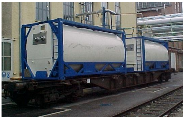
Figure 30: Railway wagon with a latent heat storage system (Source: TransHeat GmbH)
