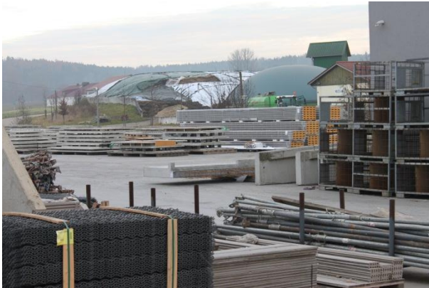
Figure 34: Heat from a biogas plant (background) in Germany supplying heat to a precast concrete factory (front) (Source: Rutz)
