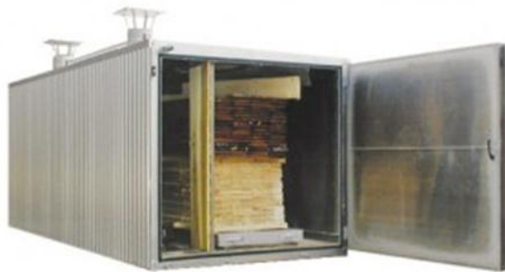
Figure 50: Example of a construction wood drying container (Source: http://www.lauberholzrockner.de )
