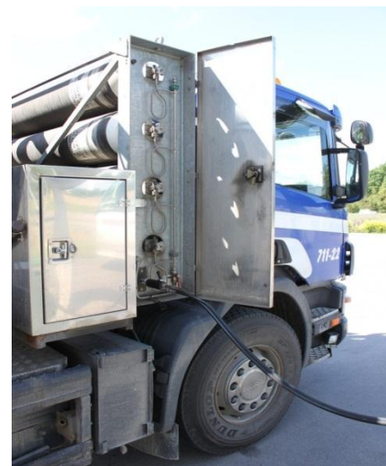
Figure 71: Tank for CBG of a truck, Sweden (Source: Rutz)
