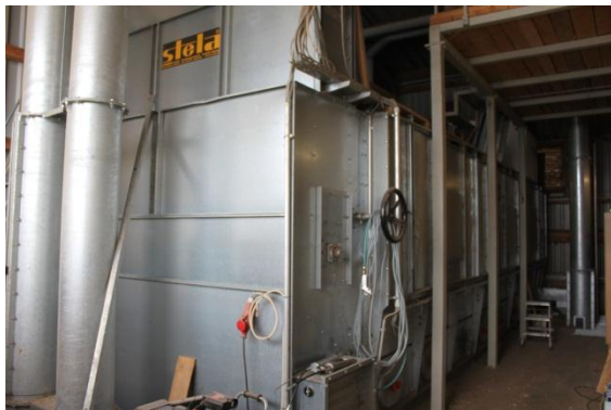
Figure 42: Feed-and-turn drier in Germany (Source: Rutz)
