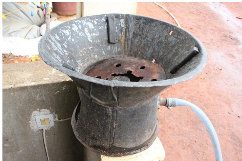
Figure 1: Biogas burner in Austria (Source: Rutz) Figure 2: One of the simplest applications for biogas: biogas stove for cooking in Mali (Source: Rutz)
