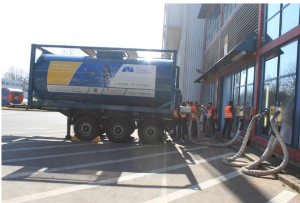
Figure 32: Heat storage container on a trailer at a waste incineration plant (Augsburg, Germany) (Source: Rutz)
