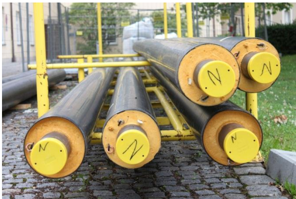
Figure 18: Insulated steel pipes for district heating in Germany (Source: Rutz)
