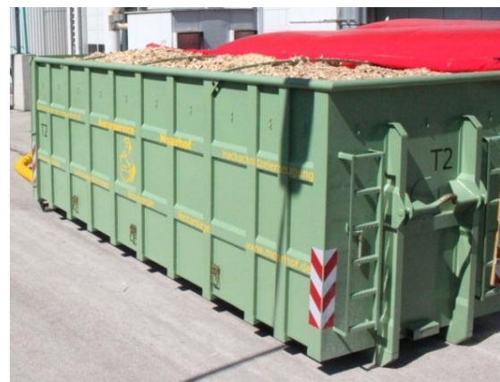
Figure 47: Container for wood chip drying in Munich, Germany (Source: Rutz)
