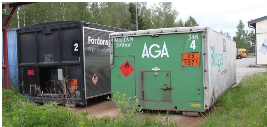
Figure 68: Containers for the transport of CBG of the biogas plant in Borås, Sweden (Source: Rutz)
