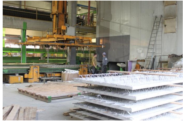
Figure 35: Precast concrete elements (front) are just removed from the drying chamber (background) (Source: Rutz)
