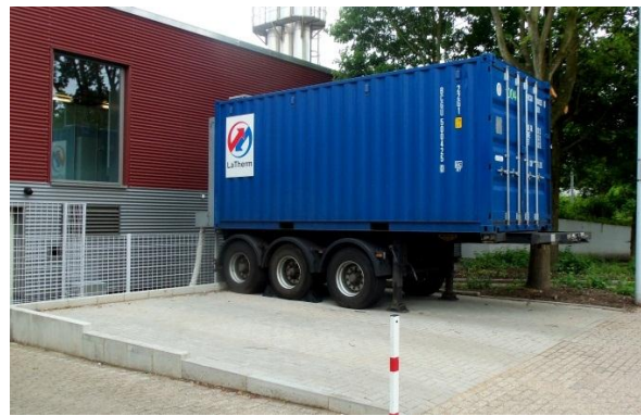
Figure 31: Trailer with a container and a latent heat storage system (Source: LaTherm GmbH)
