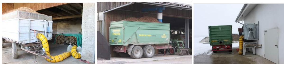
Figure 37: Examples of simple charge driers for woodchips on trailers (Source: Rutz)
