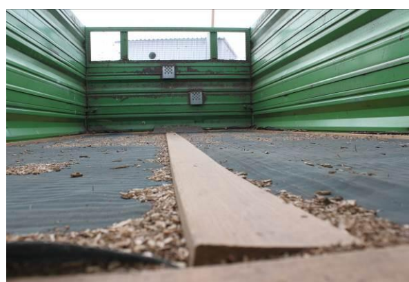
Figure 39: Own constructions of a charge drier with a perforated double-floor (Source: Rutz)
