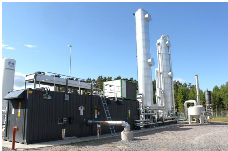
Figure 67: Water scrubber upgrading plant of Swedish Biogas International at Lidköping, Sweden (Source: Rutz)
