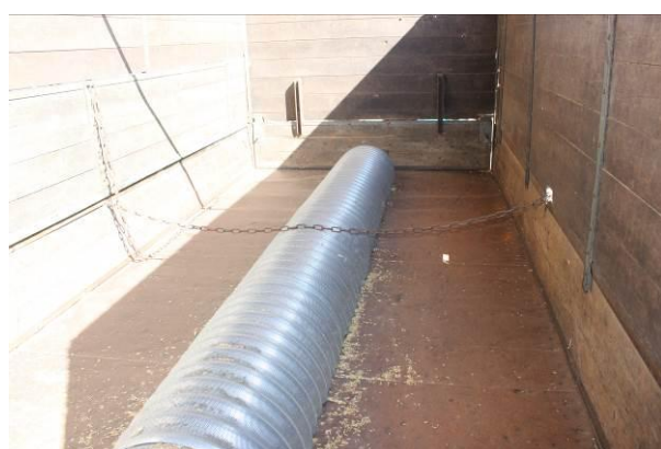
Figure 38: Own constructions of a charge drier with a perforated metal pipe (Source: Rutz)
