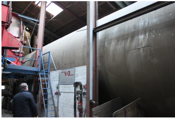
Figure 40: Drum drier for drying grass in Germany (Source: Rutz)
