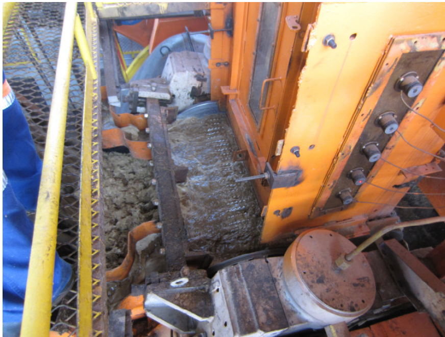
Figure 15: First mill in the process of sweet sorghum juice extraction (© Braconnier)
