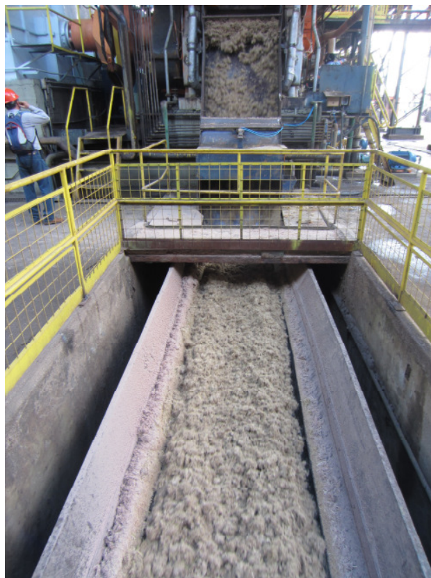
Figure 16: Bagasse left after juice extraction (© Braconnier)
