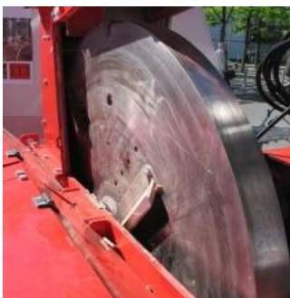
Flywheel with chipping knife of a disc-chipper ©greengain
