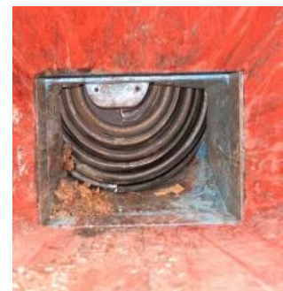
View into the grinding device of a screw-chipper ©greengain
